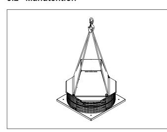
All identified fan lifting points are used to support weight and ensure safe transport via hoists, sling, spreader bar as appropriate, without damage. Maximum included angle of any support sling must not exceed 30°.
