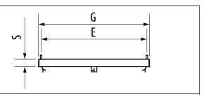
Embed the sealing frame in the built up-stand and ensure that the fixing feet are correctly embedded in the cement base.
